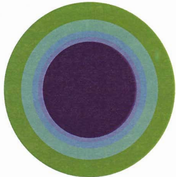
Surface Colors, psi (approximated) -45 -40 -35 -30 -25 -20 -15 -10 -5 0 5 10 15 20 25 30 35 40 45+ Standard nozzle bottom-hole pressure profile. Standard nozzles do not produce a negative pressure zone.
