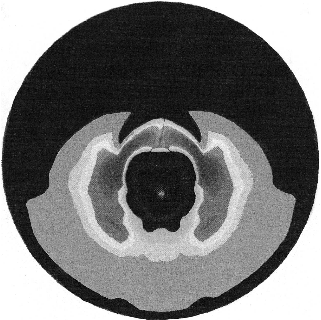
Fig. 6. Impingement pressure contours for the “Fluted Cone” include regions of less than hydrostatic pressure.
